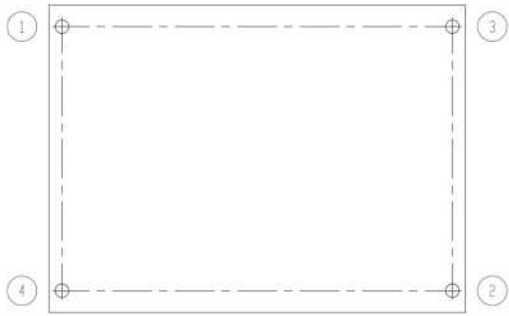
Figure 4-3 Bolts installation order (example)
