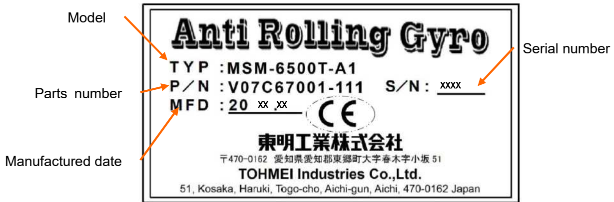
Figure 2-6 Nameplate for the ARG unit
