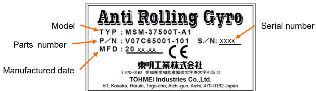
Figure 2-7 Nameplate for the ARG unit
