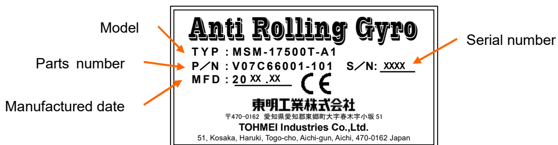
Figure 2-6 Nameplate for the ARG unit
