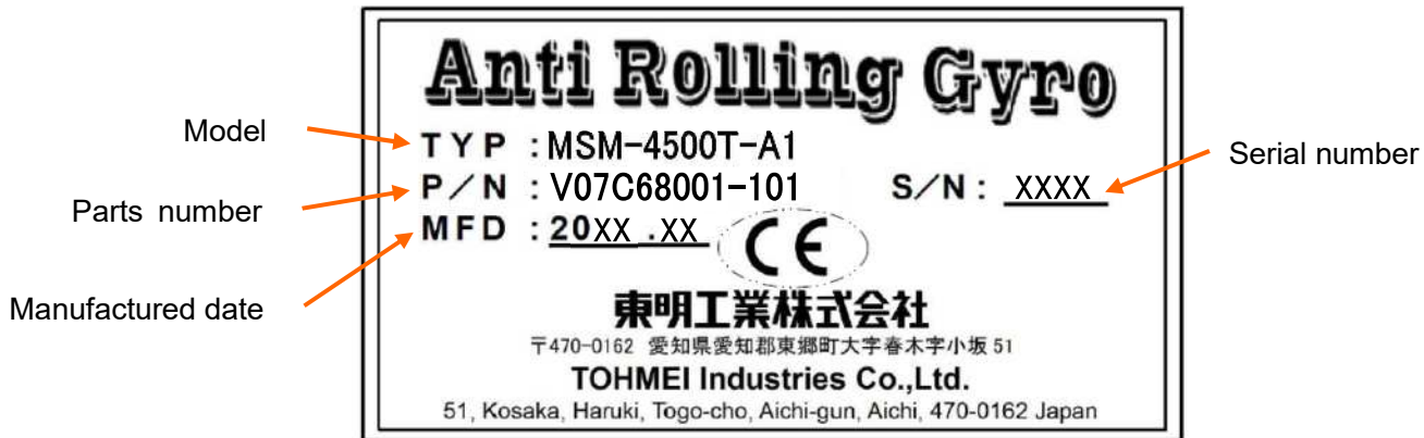
Figure 2-6 Nameplate for the ARG unit
